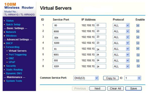
Figure 8-1 Port Mapping on Router
